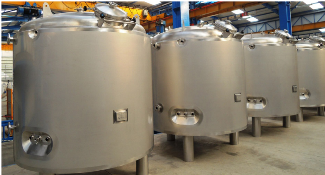
Vessels custom designed for low ceiling cleanrooms.
