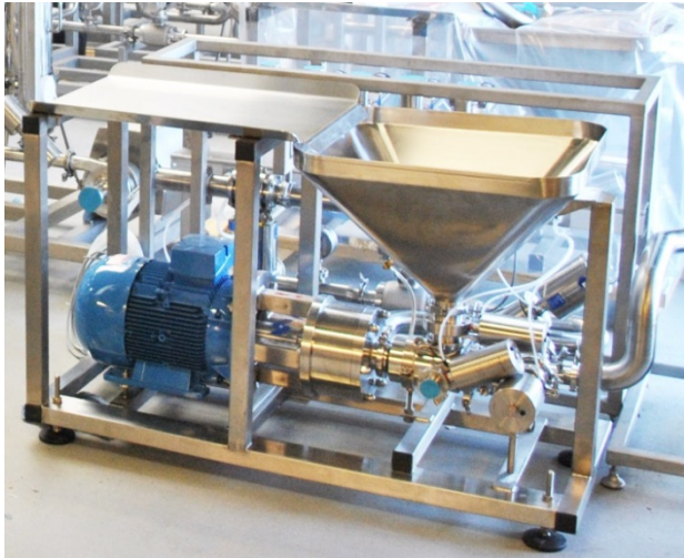
The ergonomically designed hopper eliminates the need for platforms to feed ingredients into the vessel using the manway.
